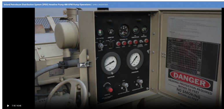
600 GPM Pump Control Panel TM Illustration and Digital Interactive Model
