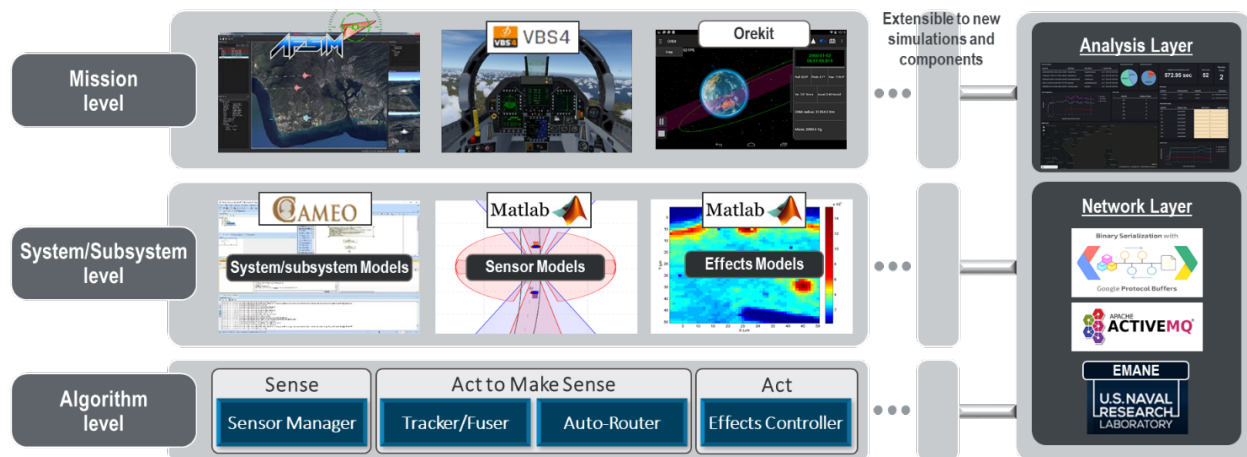
Figure 4. The JADO testbed components and architecture bridging simulation at the mission, system/subsystem and algorithm levels
