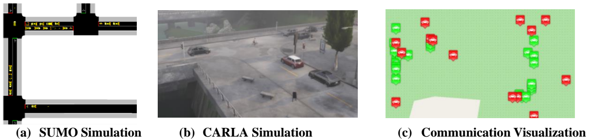
Figure 6. Simulation Demonstration: (a) SUMO Simulation; (b) CARLA Simulation; (c) Communication Visualization (red car icon shows vehicles sending V2X messages and green car icon means vehicles receiving V2X messages.)
