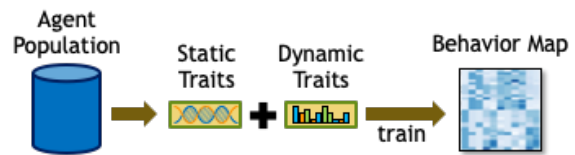
Figure 3. Constructing a Behavior Map. Behavior Maps are neural networks trained using the traits of the Agent Population.
