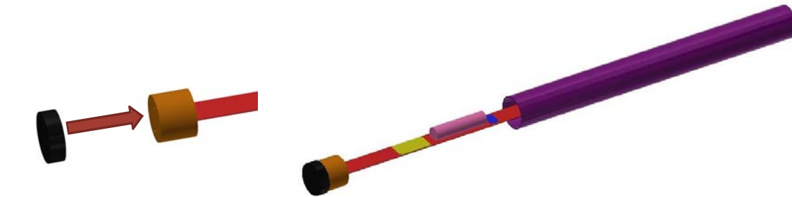
Figure 6: Insertion of frame with components into the pipe and securing the assembly with end cap
